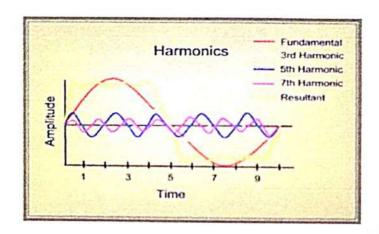
While diodes, silicon controlled rectifiers, PWM systems, thyristors, induction and are furnaces are also deployed for various requirements and due to their varying impedance characteristic, these Non Linear devices cause distortion in voltage and current waveforms which is of increasing concern in recent times. Harmonics occurs as spikes at intervals which are muptiples of supply frequency and these distort the pure sine wave form of supply voltage & current.
