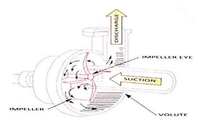
A centrifugal pump is of a very simple design. The two main parts of the pump are the impeller and the diffuser. Impeller, which is the only moving part, is attached to a shaft and driven by a motor. Impellers are generally made of bronze, polycarbonate, cast iron, stainless steel as well as other materials. The diffuser (also called as volute) houses the impeller and captures and directs the water off the impeller.
